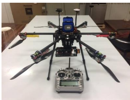
Figure 2 Unmanned Aerial Vehicle Version VESPA HEX 650 (HG Robotic company)
