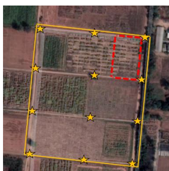
Figure 5 The position of the ground control points panel and storage
