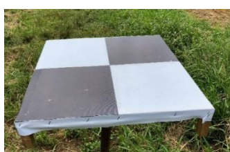
Figure 4 Ground control points panel
